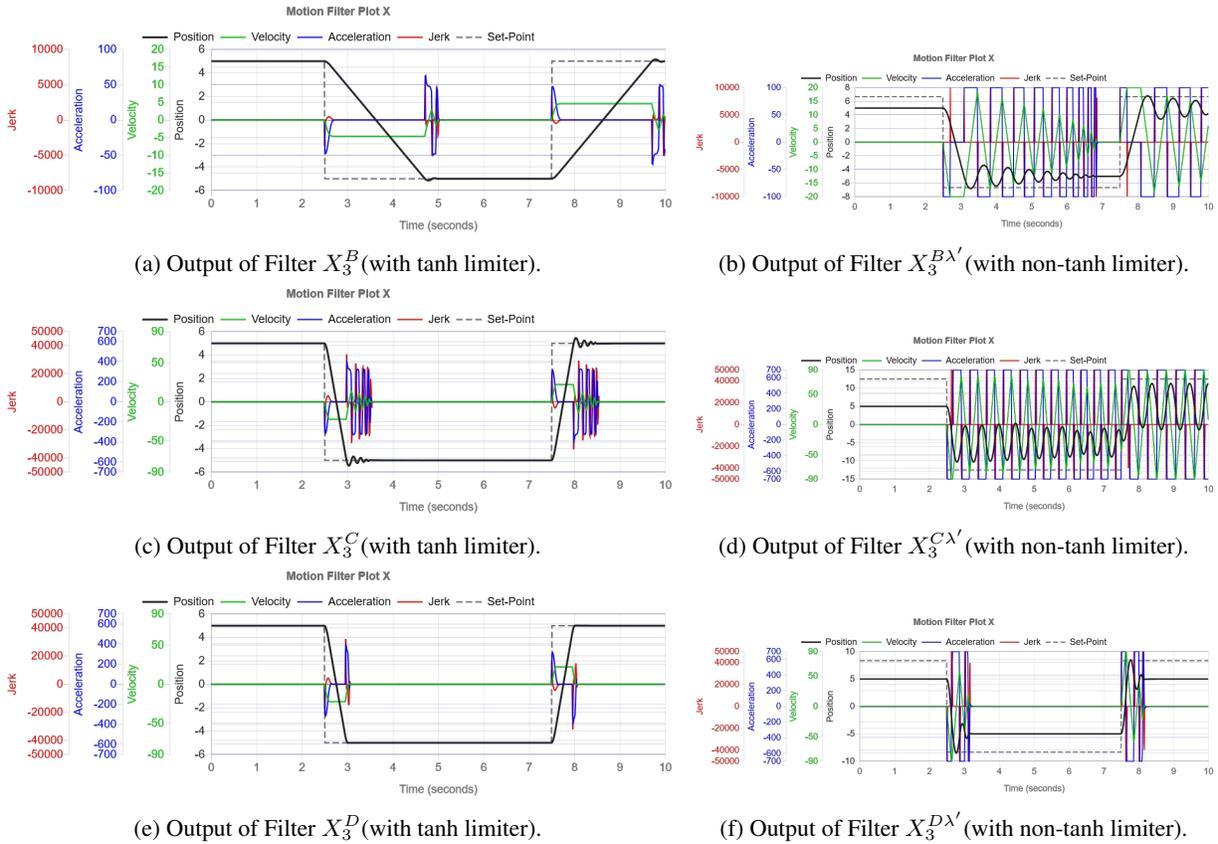
Figure 30: Output of the  $3^{rd}$  order filter of groups  $B$ ,  $C$  and  $D$ , using the *simple* input signal  $\Phi_L$ .
