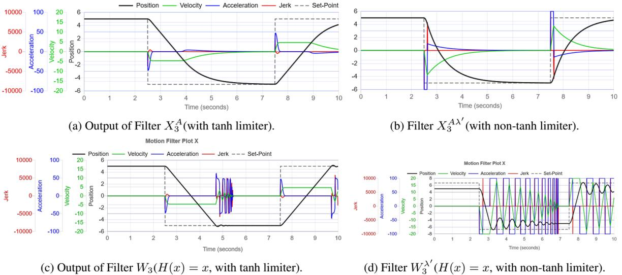
Figure 29: **Top row:** The output of filter  $X_3^A$  (a) compared to filter  $X_3^{A\lambda'}$  (b). **Bottom row:** The output produced by the NMF equations if the transfer function was bypassed, i.e., making  $H(x) = x$ , while using the tanh-based limiter on the left (c), and a non-tanh based limiter on the right (d). All four plots are produced from the *simple* input signal  $\Phi_L$ .
