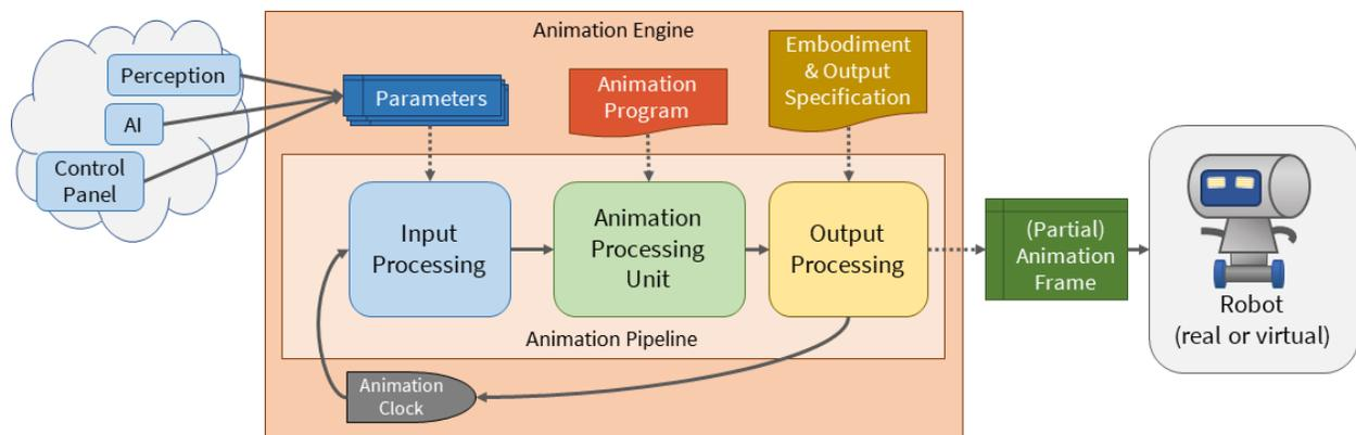
Figure 23: A *Nutty*-based animation engine, including the *Nutty Pipeline*. At each clock cycle, the Input parameters along with the selected Animation Program are provided to the Animation Program Processor, which outputs a (Partial) Animation Frame contains the motion parameters for each programmable DoF.
