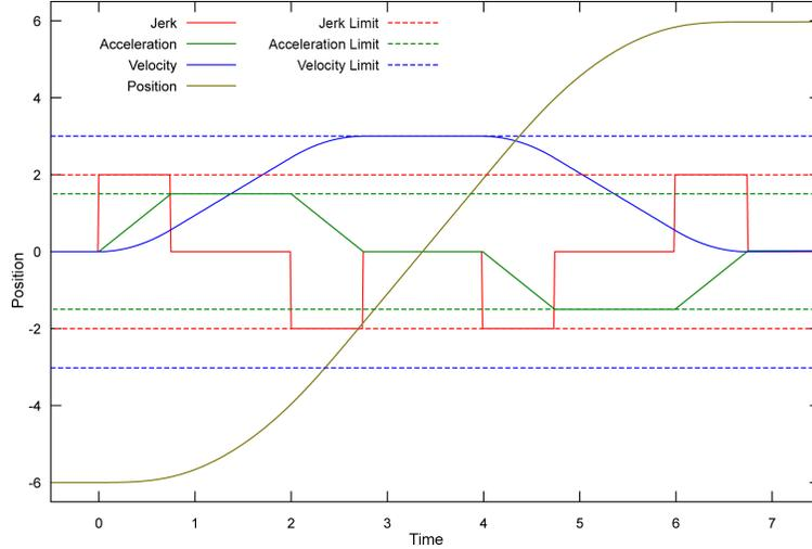
Figure 25: A diagram illustrating jerk, acceleration and velocity of a  $C^3$  continuous motion signal that moves from -6 to 6.<sup>14</sup>
