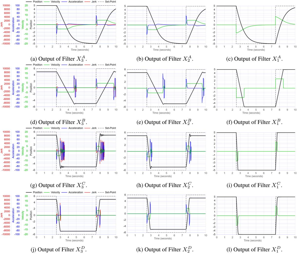
Figure 31: Comparison of the  $3^{rd}$ ,  $2^{nd}$  and  $1^{st}$  order filters for hyperparameter groups  $A$  (first row),  $B$  (second row)  $C$  (third row) and  $D$  (last row), using the *simple* input signal  $\Phi_L$ .
