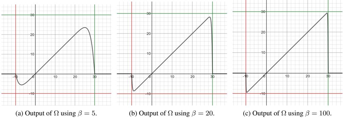
Figure 26: Comparison of the output saturation function  $\Omega$  given the minimum and maximum limits of  $[-10, 20]$ , using three different exponents  $\beta \in [5, 20, 100]$ .
