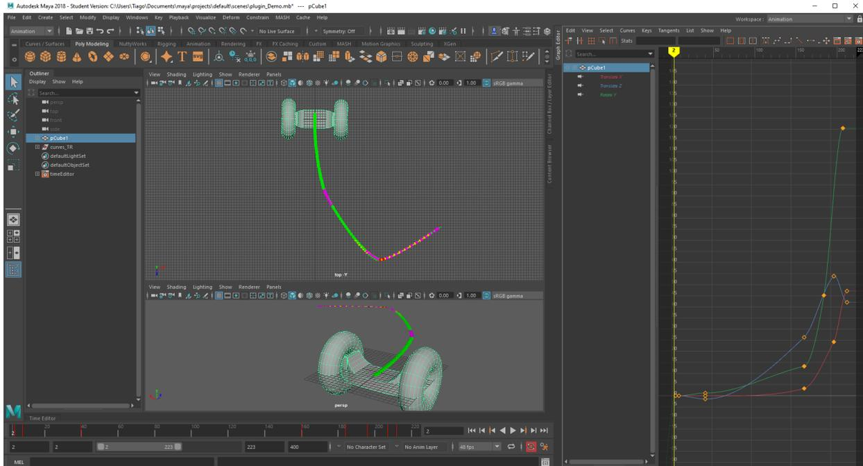
Figure 35: A screenshot illustrating the robot-animation trajectory-helper feature implemented through a plug-in into Autodesk Maya. This feature draws the motion trajectory as a path directly into the scene of the animation software, and highlights the points of the trajectory that break any of the robot’s kinematic limits.
