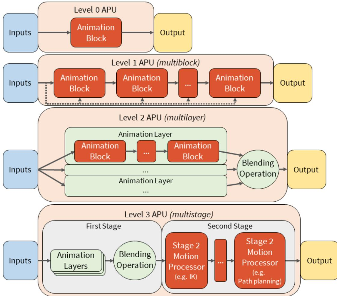
Figure 24: The four types of *Nutty* APUs.
