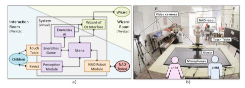
Fig. 1. a) Real environment setup. b) System architecture
